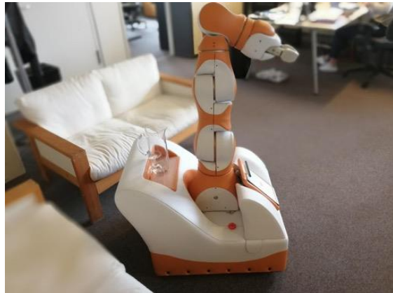
Personal Service Assistant Lio, including P-Rob and a sophisticated sensor equipped mobile platform
