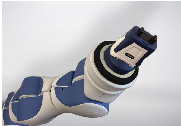
P-Rob with ISO normed gripper connector and SCHUNK collaborative parallel gripper
