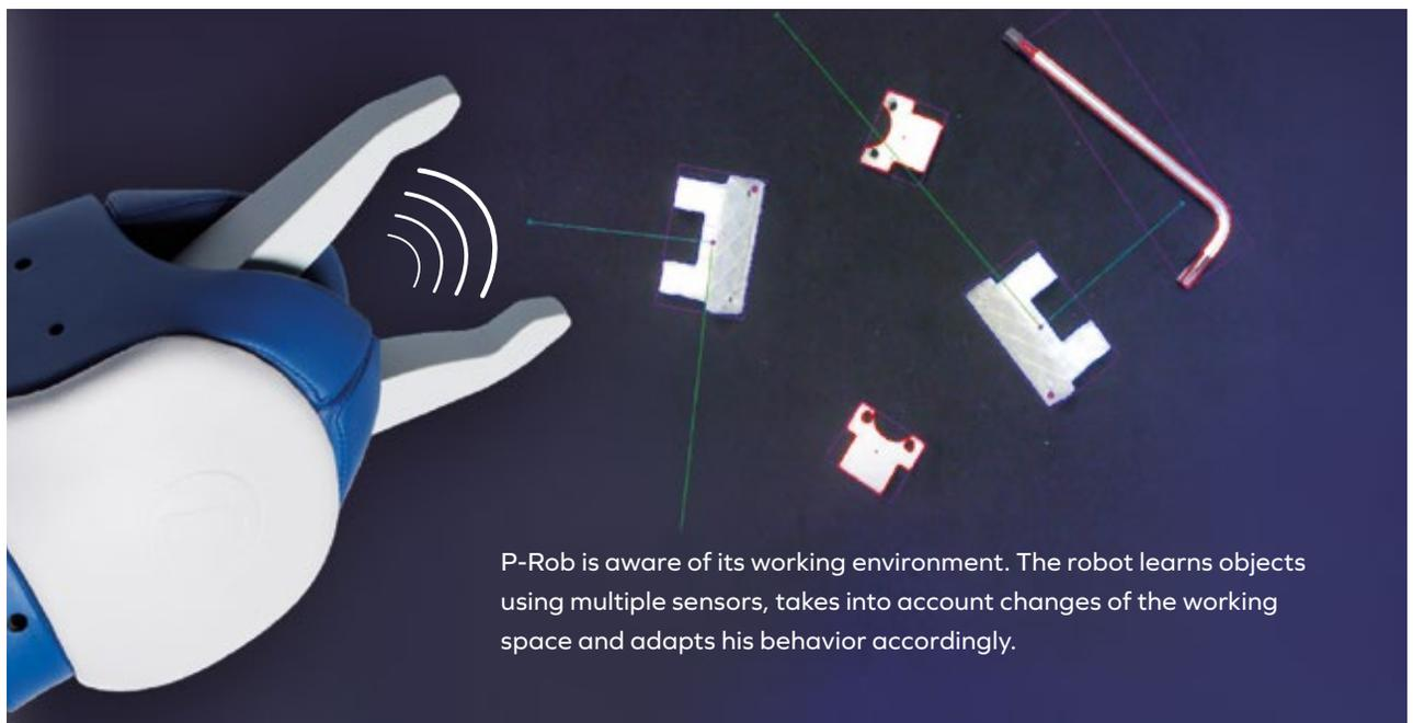
P-Rob is aware of its working environment. The robot learns objects using multiple sensors, takes into account changes of the working space and adapts his behavior accordingly.
